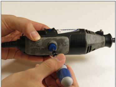
• Remove the blue caps located on either side of the MultiPro, using a <u>3 mm flathead</u> screwdriver.
