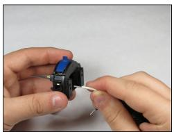
• Remove the 2 wires on the back of the switch, connecting the cord to the switch, by inserting a small metal pick into the hole next to the wires and pulling the pick and the wire out together.
