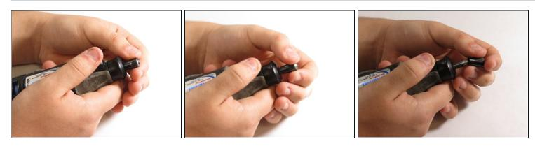
• Hold down the collet lock, remove the chuck cap from the top of the Multipro by screwing counterclockwise.
