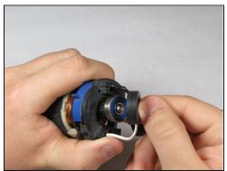
• Remove the rubber ring from the bottom of the armature.
