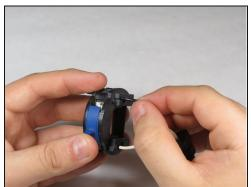
• Carefully insert the wires into the new switch making sure the white wire is attached to left hand side and the black wire is attached to the right hand side when the switch is facing up. By pushing the wires in with your hand.
