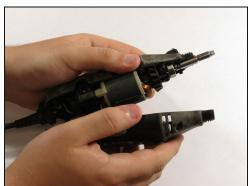
• Pull the bottom side of the casing up to remove it.
