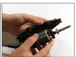
• Gently lift the motor shaft out of the Multipro.
