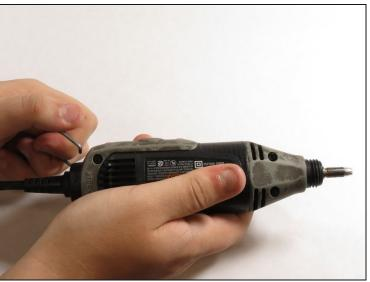
• Pull one side of the hanger up and then pull away from the Multipro until the other side can be pulled out.
