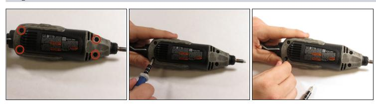
• Remove the 4 15mm screws located on the bottom of the Multipro with a T-15 screwdriver.
