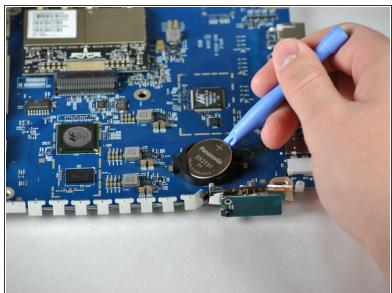
Wedge the tip of a plastic opening tool between the battery and the securing clip. Pop the battery out using sufficient leverage.
