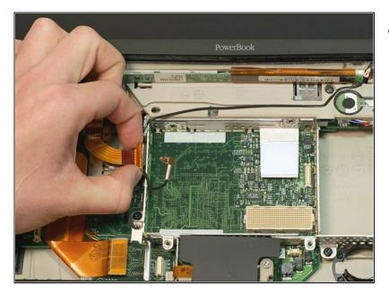
Grasp the orange display data cable and disconnect it from the logic board.
