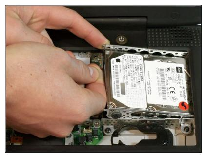
Grasp the plastic tab and pull the hard drive up and to the left, making sure that the metal bracket doesn't catch on the black plastic casing.
