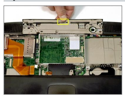
• Grasp the upper plastic casing where it locks into the internal frame and pull back. When the plastic tab has cleared the slot that the casing locks into, pull up enough to keep it from locking back into place.
