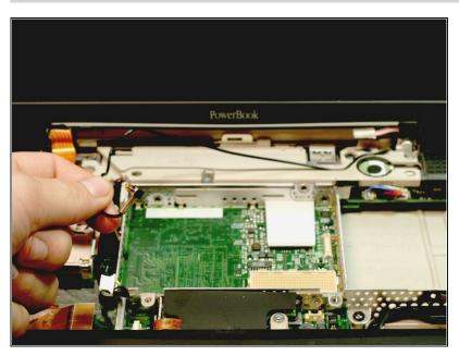
• Returning to the front, pull the black Airport antenna up from its recessed housing.
