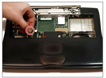
• Disconnect the wide orange cable that connects the airport card slot to the logic board.
