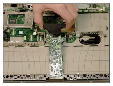
• Grasp the power card near the black shield and lift up.
