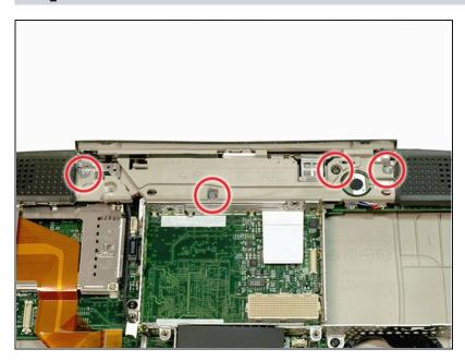
Remove the three long silver and one short black Torx screws from the beige plastic casing.
