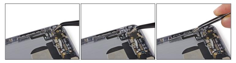
• Pull the hold switch and volume control button brackets away from the rear case to allow access to the button covers.
