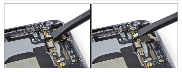
• Use the flat end of a spudger to lift the volume control cable connector up off of its socket.
