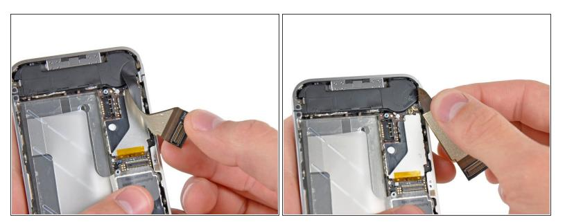
• Carefully peel the dock ribbon cable off the logic board and the lower speaker enclosure.
