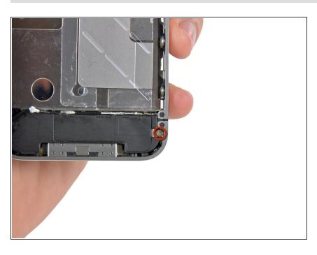
Remove the single 2.4 mm Phillips screw securing the speaker enclosure to the side of the inner frame.
