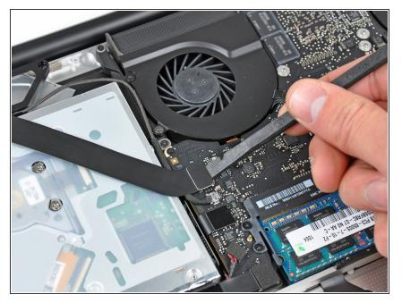
Use the flat end of a spudger to carefully pry the AirPort/Bluetooth ribbon cable up off its socket on the logic board.
