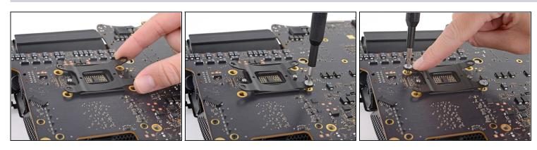
• Place the spring plate on the backing plate.
