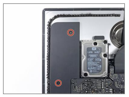
Remove two 10 mm T10 screws.
