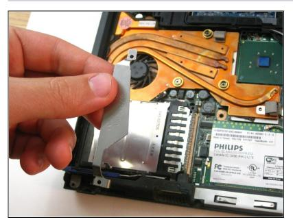
• Lift the bracket up and out.
