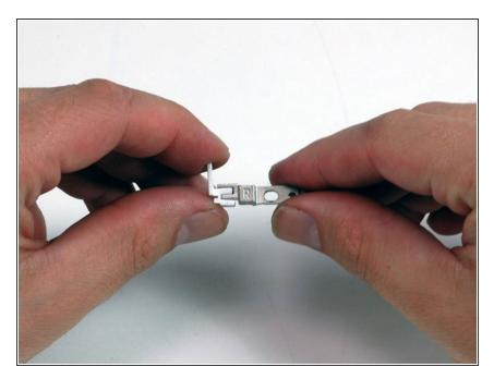
• Slide the plastic dust cover out of its slot in the right hinge mount.
