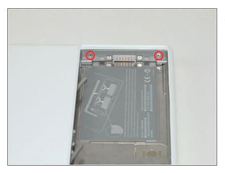
Remove the two 6 mm Phillips #00 screws from either side of the right wall of the battery compartment (not the ones closest to the battery connector).
