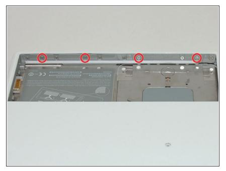
Remove the four 3 mm indicated Phillips #00 screws from the front wall of the battery compartment.
