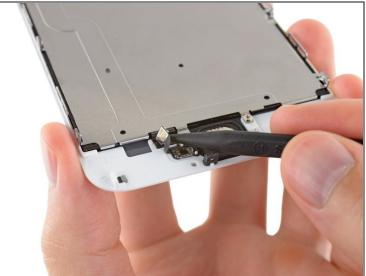
• Use the tip of a spudger to disconnect the home button connector from its socket on the home button cable.
