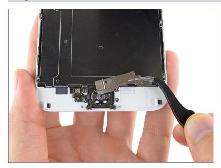
Remove the home button bracket from the front panel assembly.
