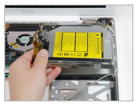
Lift the front edge of the optical drive and slide it up and out of the computer.
