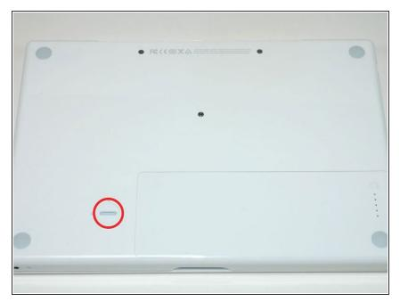
Use a coin or spudger to rotate the battery-locking screw 90 degrees clockwise.
