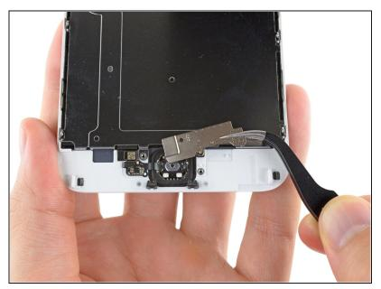
Remove the home button bracket from the front panel assembly.
