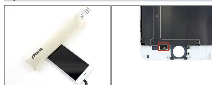
(i) The next step requires peeling one end of the home button cable (highlighted in red in the second picture) that is affixed to the back of the display assembly with strong adhesive. We highly recommend <u>using an iOpener</u> to heat the bottom of the display assembly, directly on top of the home button.
