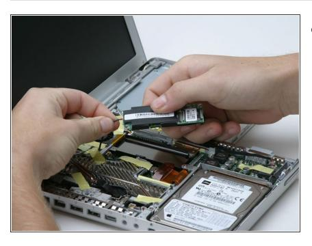
Disconnect the modem cable from the modem.
