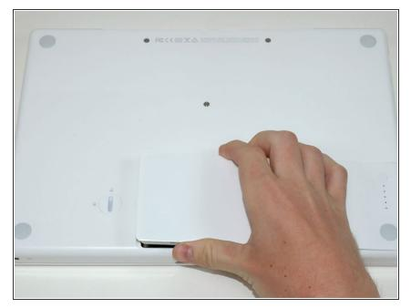
Lift the battery out of the computer.
