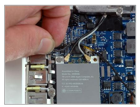
Deroute the left speaker cable from beneath the Airport antenna cables.
