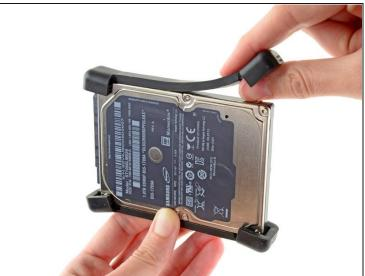
• Peel the rubber hard drive bumpers up off the top and bottom edges of the hard drive.
