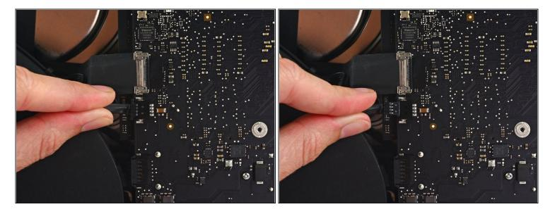
• Pull the fan cable connector straight away from its socket on the logic board.
