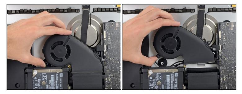
• Lift and remove the fan from the iMac.
