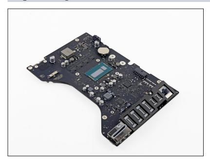
During reassembly of the logic board, pay attention to the position of the I/O connectors.
