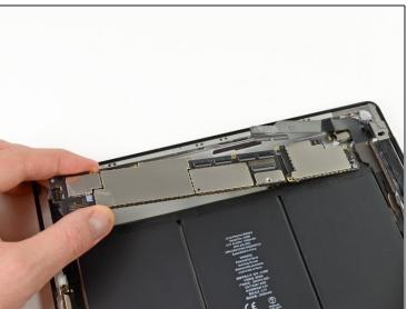
• Holding the logic board by the side nearest the dock connector, carefully pull the logic board toward the bottom of the iPad.
