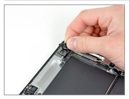
• Carefully peel the rubber cover off the metal camera retainer and remove it from the iPad 2.
