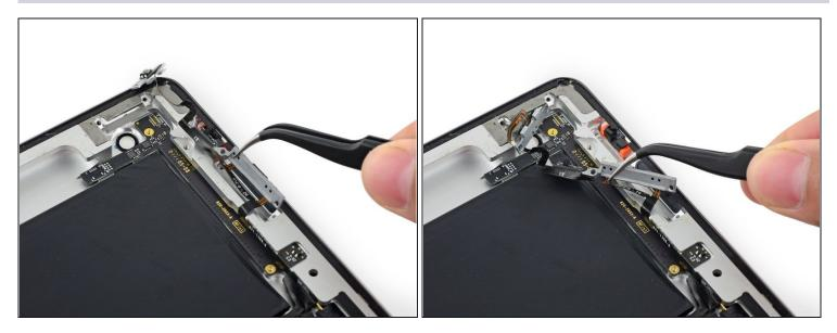
• Bend the cable toward the inside of the rear case, but **do not attempt to remove it** as it is still connected to the upper component board.
