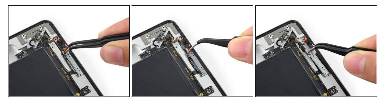
• Use the center screw hole of the volume control bracket to tilt it out toward the edge of the case and then pull it up out of its recess.
