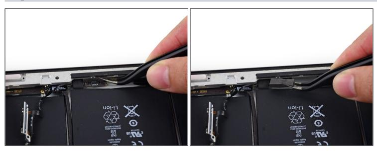
• Use a set of tweezers to remove the foam block from between the rear case and the upper component board.
