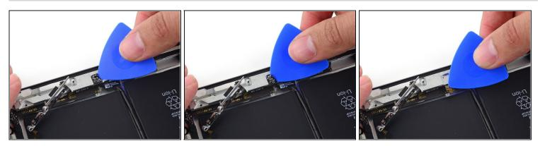
• Use the point of an opening pick to gently peel the Smart Cover sleep/wake sensor up off the rear case.
