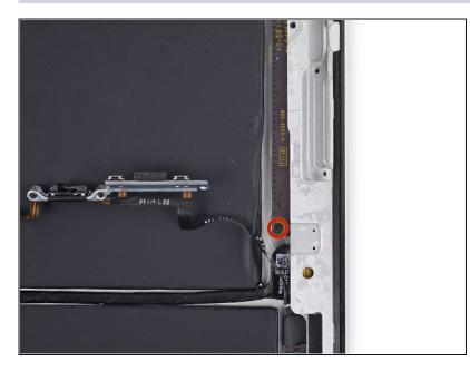
Remove the single 2 mm Phillips #000 screw from the lower end of the upper component board.
