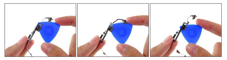
• Slide the opening pick under the remaining portion of the rotation lock/silent switch to peel it up off the button bracket.
