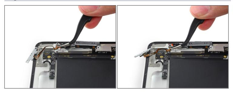
• Gently lift the cable between the power button and volume rocker up off of the rear case.
