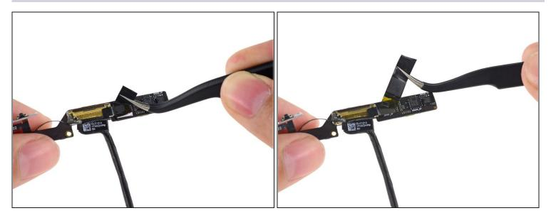
• Peel the tape covering the button cable connector off of the upper component board.
