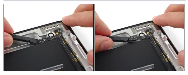
• Insert a spudger under the upper left end of the upper component board and lift it up off of its adhesive.
