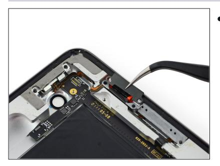
Remove the metal bracket securing the rotation lock/silent switch.
