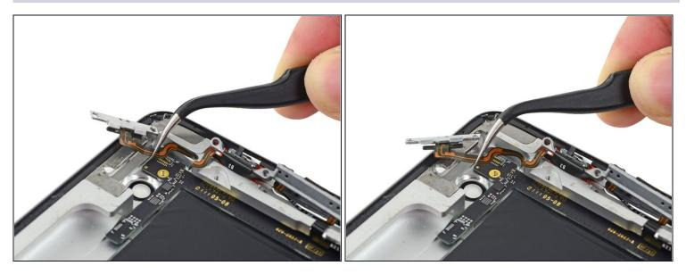
• Gently peel the power button portion of the cable away from the rear case.
