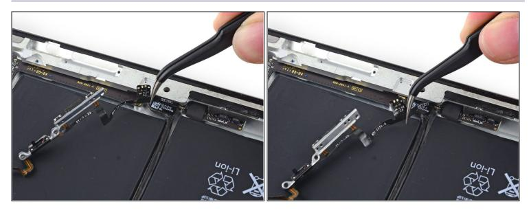
• Gently peel the last vertical portion off of the rear case.
