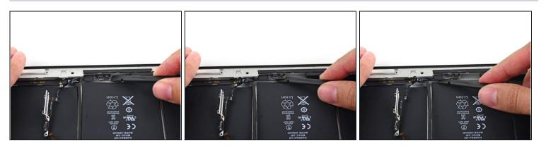
• Insert a spudger under the end of the upper component board and gently slide it toward the volume rocker to free the board from adhesive.
