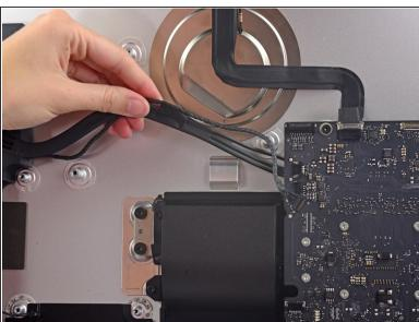
In a similar fashion as the previous step, de-route the combo SATA data/power cable up out of the retaining clip.
