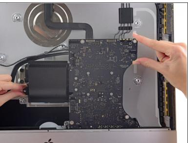
Tilt the top of the logic board away from the rear enclosure.
