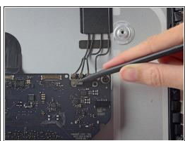
(i) If necessary, use the tip of a spudger to peel back the tabs covering the antenna connectors.
