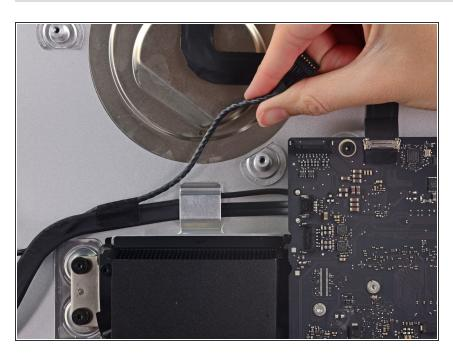
De-route the left speaker cable by pulling it straight up out of the retaining clip in the back of the rear enclosure.
