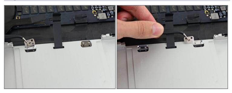
• Use tweezers to remove the two trackpad mounting brackets from the upper case.
