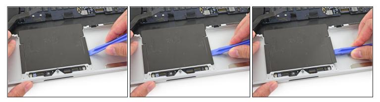
• Use a plastic opening tool to carefully pry the trackpad cover plate up from the upper case.
