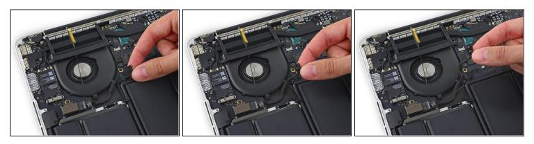
• Carefully peel the right speaker cable off the upper case.
