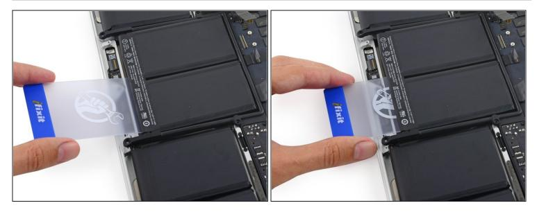
• Pull the card back out and insert it about an inch between the right-center battery cell and the upper case, separating the adhesive between the cell and case.
