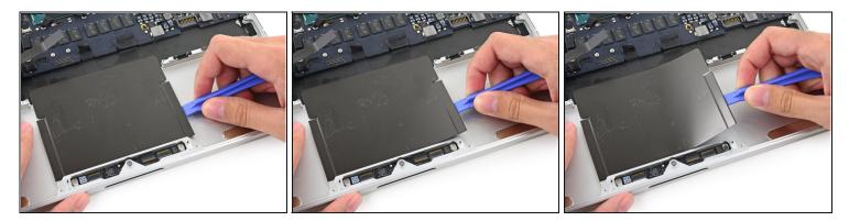
• Use a plastic opening tool to slowly and carefully peel the trackpad cover plate up off the upper case.
