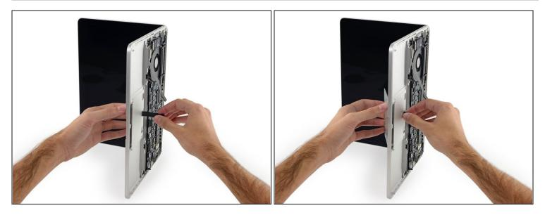
🗷 To avoid scratching the display, open the computer about 90° and set it on end.
