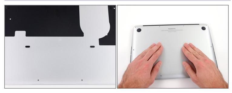
i The lower case is connected to the upper case with two plastic clips near its center.
