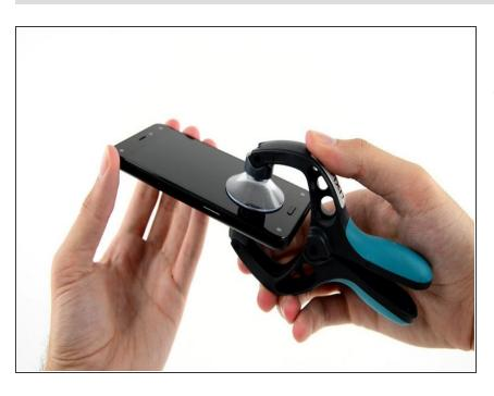
No glass sealing will keep us out of this phone. With the screws out of the way, it's time to turn up the heat.
