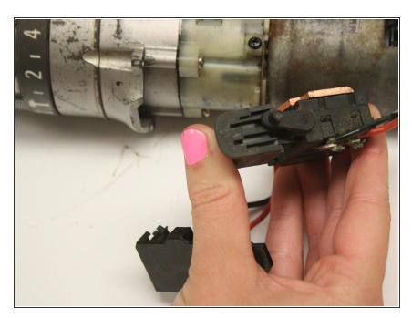
Make sure plastic is not broken and switch is not stuck.
