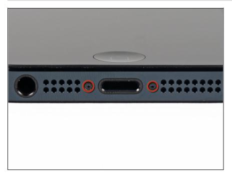
• Use the Pentalobe screwdriver to remove the two 3.6 mm Pentalobe screws near the dock connector.
