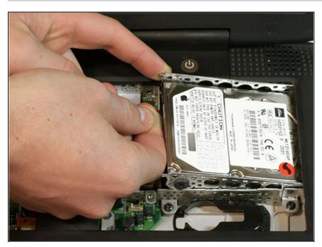
Grasp the plastic tab and pull the hard drive up and to the left, making sure that the metal bracket doesn't catch on the black plastic casing.
