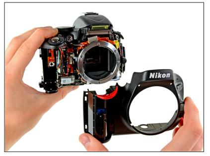
Firmly separate the front panel from the main camera body.
