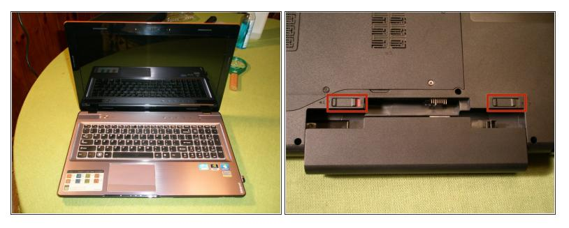
From the bottom of the unit: Slide the 2 latches to the outer edges and remove the battery.
