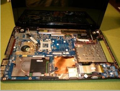
Using a plastic pry tool or guitar pick, carefully unsnap the top bezel and remove it.
