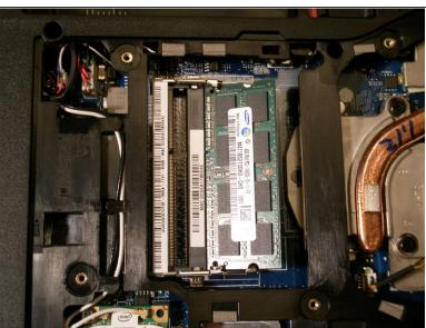
Push the retaining clips on both sides of the DIMM memory cards to release and remove them from the unit.
