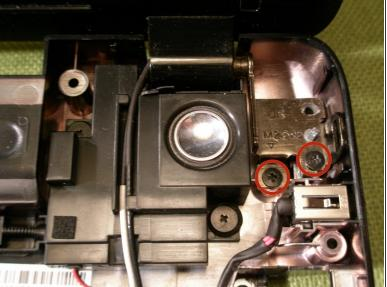
Remove the 3 remaining screws on the LCD hinges and carefully lift the LCD unit from the chassis.
