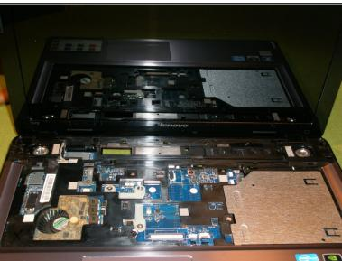
Using a plastic pry tool or guitar pick, carefully unsnap and lift the power button/status LED cover and remove it.
