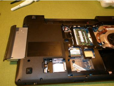
• Remove the 1 retaining screw from the optical drive and slide it out of the unit.
