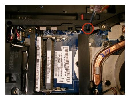
Remove the single keyboard retaining screw. This screw and the screw that held the optical drive in place also attach to the back of the keyboard.
