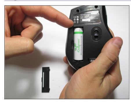
• Remove the battery with a finger nail or a nonmetal tool.
