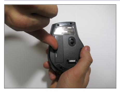
Remove the battery cover with a plastic opening tool, nylon spudger, or a fingernail.
