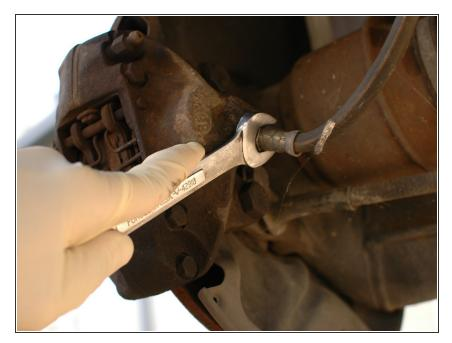
With the upper connection free, now loosen the connection of the soft rubber hose at the caliper. This is done with a 14mm open-end wrench.
