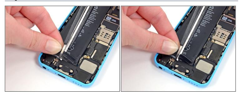
• Cut the black battery adhesive tab between the two white adhesive strips, separating them.
