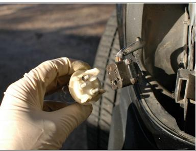
• While we have the bulb out, you can see here that the connection area between the plug and the socket is rather dirty. Use a soft metal brush such as a brass brush, and some electric contact cleaner, to clean the components. The two pictures show before and after cleaning.
