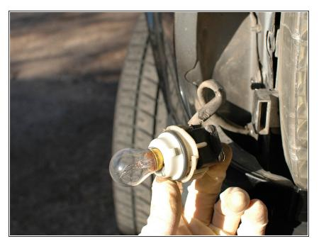
Remove the bulb from the socket by turning it counterclockwise.
