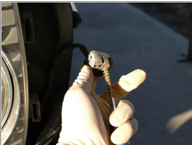
Additionally, consider using a soft metal brush such as the ones shown to clean the inside of the bulb socket as well as the insides of the plug connections to remove any corrosion.
