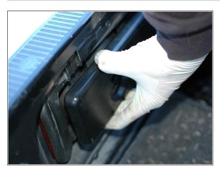
Pull the panel out and away from the back of the car, being careful not to force the bulbs out of the holes.
