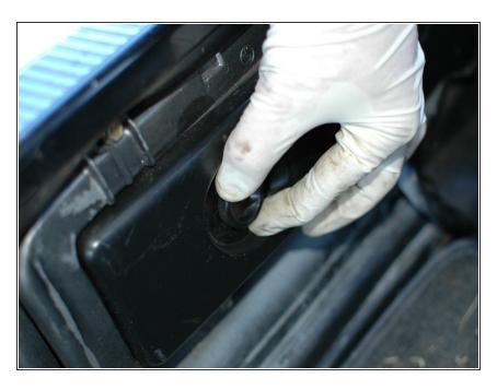
The panel is secured with two thumb screws. Remove these.
