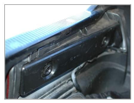
The access panel for all of these lights is on the inside of the trunk. There's one on each side. This guide will cover one side; simply repeat on the other to complete the job.
