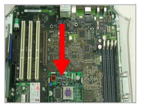
After removing the (3) #2 philips screws, remove the (4) 1/4" hex nuts, then slide as directed and remove board.
