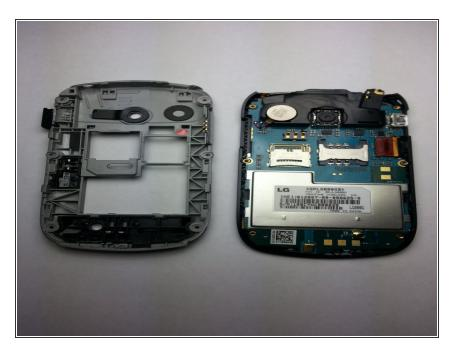
Using the plastic opening tool, pry off the shell of the phone, revealing the motherboard
