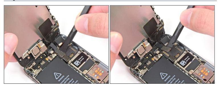
• Finally, disconnect the digitizer cable connector.
