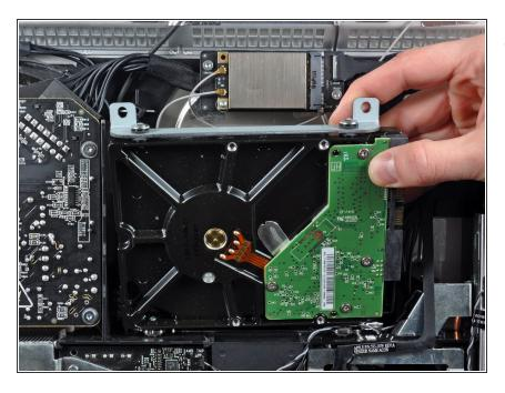
Slightly rotate the hard drive out of the outer case and lift it up off its mounting pins toward the top edge of the iMac.
