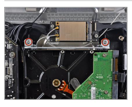
Remove the two 9 mm T10 Torx screws securing the upper hard drive bracket to the outer case.
