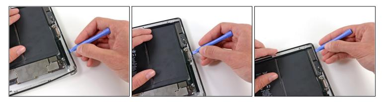
• When you get close to the bottom left edge, rotate the plastic opening tool around the corner, and continue sliding it along the bottom edge.
