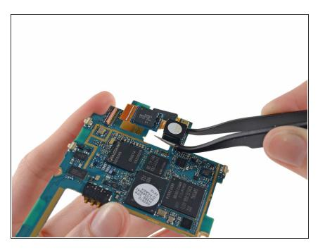
Remove the rear-facing camera from the motherboard.
