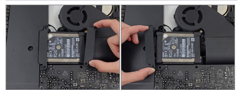
• Remove the left and right hard drive brackets from the iMac.
