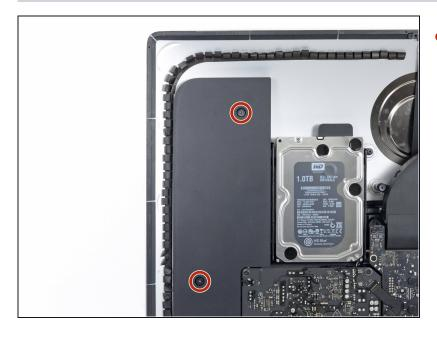
• Remove two 10 mm T10 screws.
