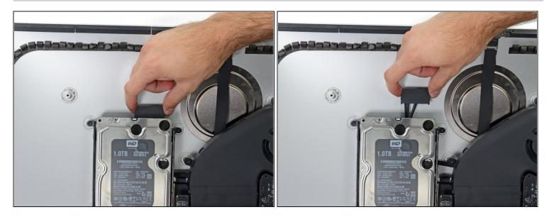
• Pull straight up on the SATA data/power cable to disconnect it from the drive.
