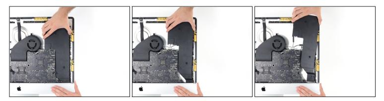
• Lift the speaker straight up and remove it from the iMac.
