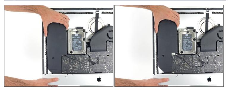
• Lift the left speaker straight up, until the power button cable is exposed (about 0.5 inches).
