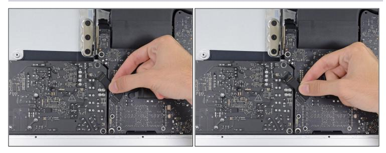
A When working on the power supply, **be very careful** not to touch the capacitor leads or any exposed solder joints on the back of the power supply. Only handle the board by the edges.
