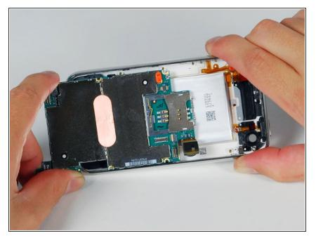
Slide the logic board towards the dock connector and out of the iPhone.
