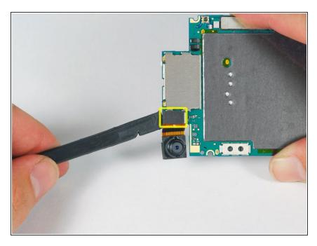
• Use a spudger to disconnect the camera from the logic board.
