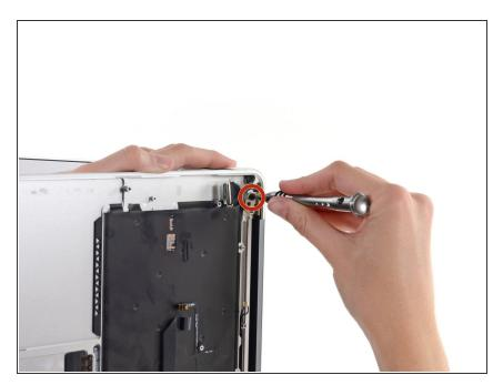
While holding the Air steady, remove the remaining 4.9 mm T8 Torx screw from the display bracket.
