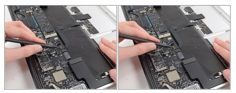
Use the tip of a spudger or your fingernail to flip up the retaining flap on the trackpad ribbon cable ZIF socket.
