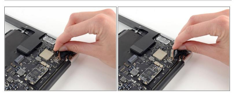
Grab the plastic pull tab secured to the display data cable lock and rotate it towards the top side of the computer.
