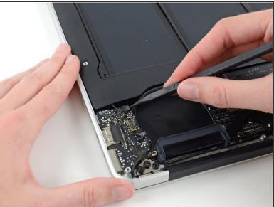
Use the tip of a spudger to carefully flip up the retaining flap on the microphone ribbon cable ZIF socket.
