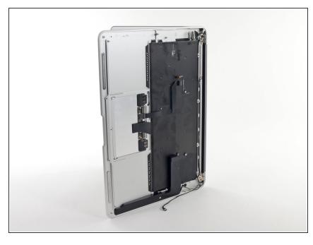
Open the display so that it is perpendicular to the upper case and place it on a table as shown.
