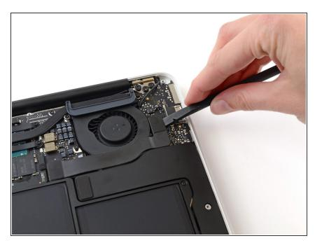
Use the flat end of a spudger to pry the I/O board cable connector up out of its socket on the I/O board.
