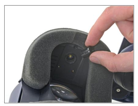
Remove the two plastic spacers underneath the previously removed screws from the headset.
