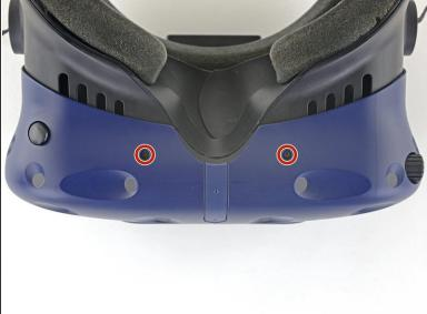
• Use a T6 Torx screwdriver to remove the four 3.9 mm screws (two on top, two on bottom) securing the outer shell to the headset.
