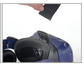
Feed the top strap through the clip on the headset to fully remove it.
