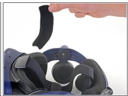
Peel off both front side foam pads to uncover the speaker wires.
