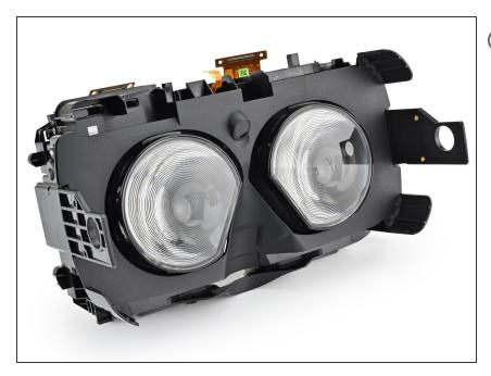
Only the lens and OLED assembly remain.
