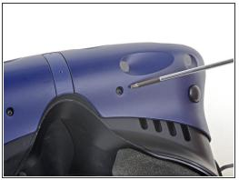
i The four screws securing the outer shell are covered with black stickers. If the stickers are difficult to remove, simply press your T6 Torx driver through them.
