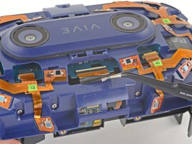
Use a pair of tweezers to peel back the grey tape covering the ZIF connector on the motherboard underneath the sensor array.
