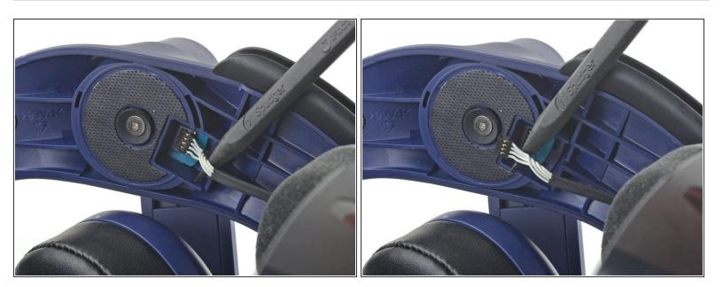
Use the pointed end of your spudger to pry up and disconnect both the left and right headphone speaker wires.
