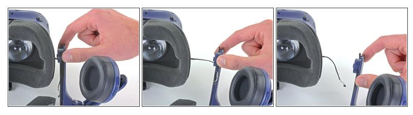
Thread the headphone speaker wires out through the ends of the head strap.
