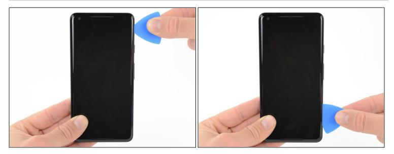
• Slide the opening pick down the right side of the phone to separate the display adhesive.
