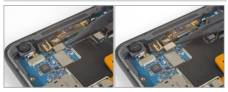
• Use the point of a spudger to disconnect the front-facing sensor assembly connector.
