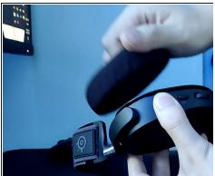
Remove the cup by inserting your four fingers in the inner ring of the cup, with your thumb softly pressing against them from the outside. Slowly turn it clockwise/counterclockwise while pulling up, and the cup should come off. If you need help doing this part, there are plenty of YouTube guides for this step, as this is universal for Arctis units.
