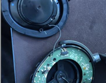
With the cup off, now you need a Torx TR6 bit to remove three screws. This is relatively easy, but do be careful when removing the lid, as there is a wire connecting it to the pcb housed in the body.
