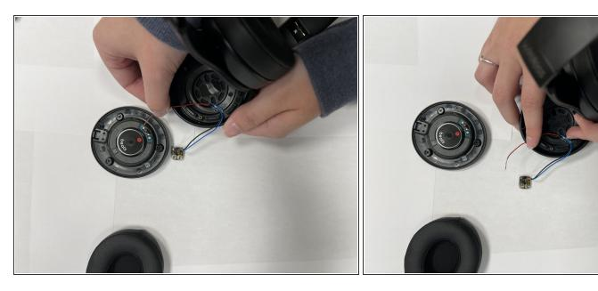
After you desolder all wires you are able to remove and replace the charging port.
