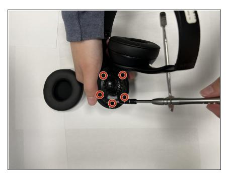
Use a Phillips #00 screwdriver to remove the five screws that hold the speaker in place.
