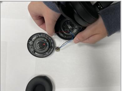
De-solder wires connecting the circuit panel to the rest of the device.
