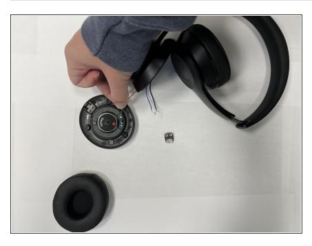
Solder wires onto the new circuit panel.
