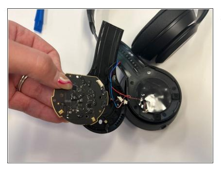
• Finally, remove and replace the motherboard.
