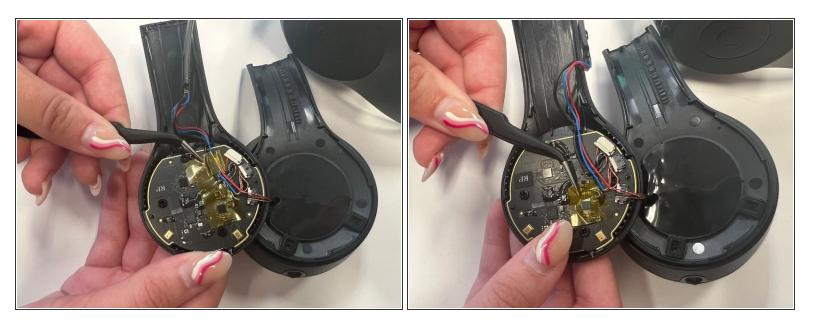
Use a pair of tweezers to carefully remove the yellow polyimide tape that is attached to the morherboard.
