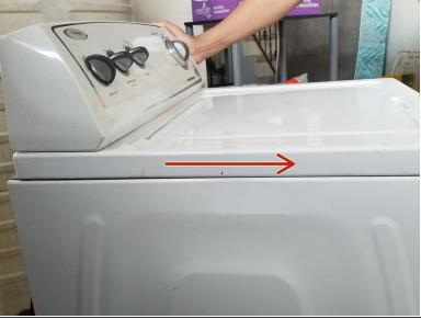
Gently pull the upper machine loading lid towards you to the to release the front latch mechanism.
