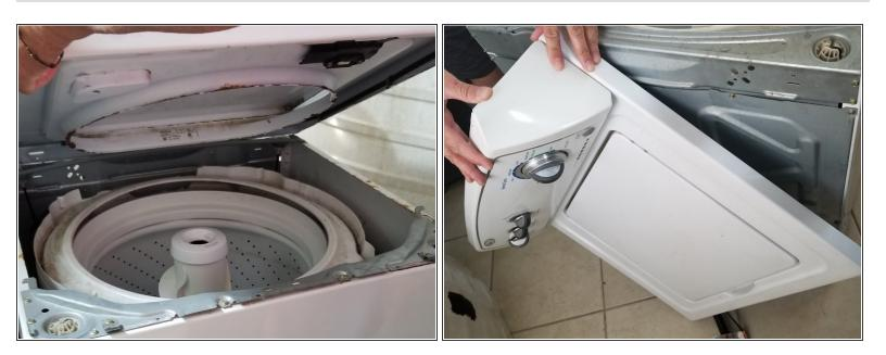
Lift the loading lid off the machine and set it down gently in a secure place.
