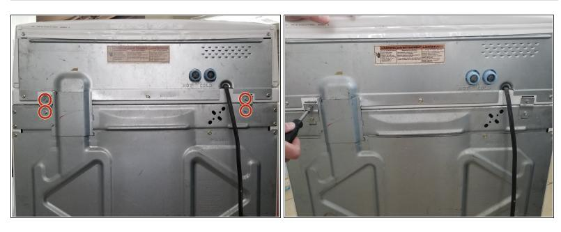
• Use an 1/4 inch nut driver to remove the four 9.5 mm hex screws on the back of the machine that secure the upper machine loading lid and console.
