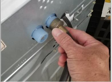
• Turn the water hose fitting counterclockwise to unplug it from the machine.
