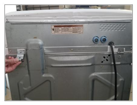
Remove the two brackets on the back by tilting them slightly upwards and then outwards.
