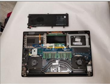
Carefully remove the battery from the computer.
